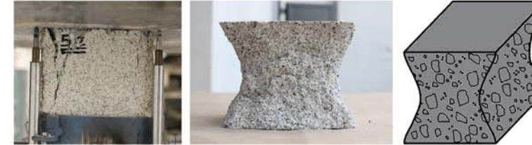
Optimal mechanical failure compared to standard UNI EN 12390-3
